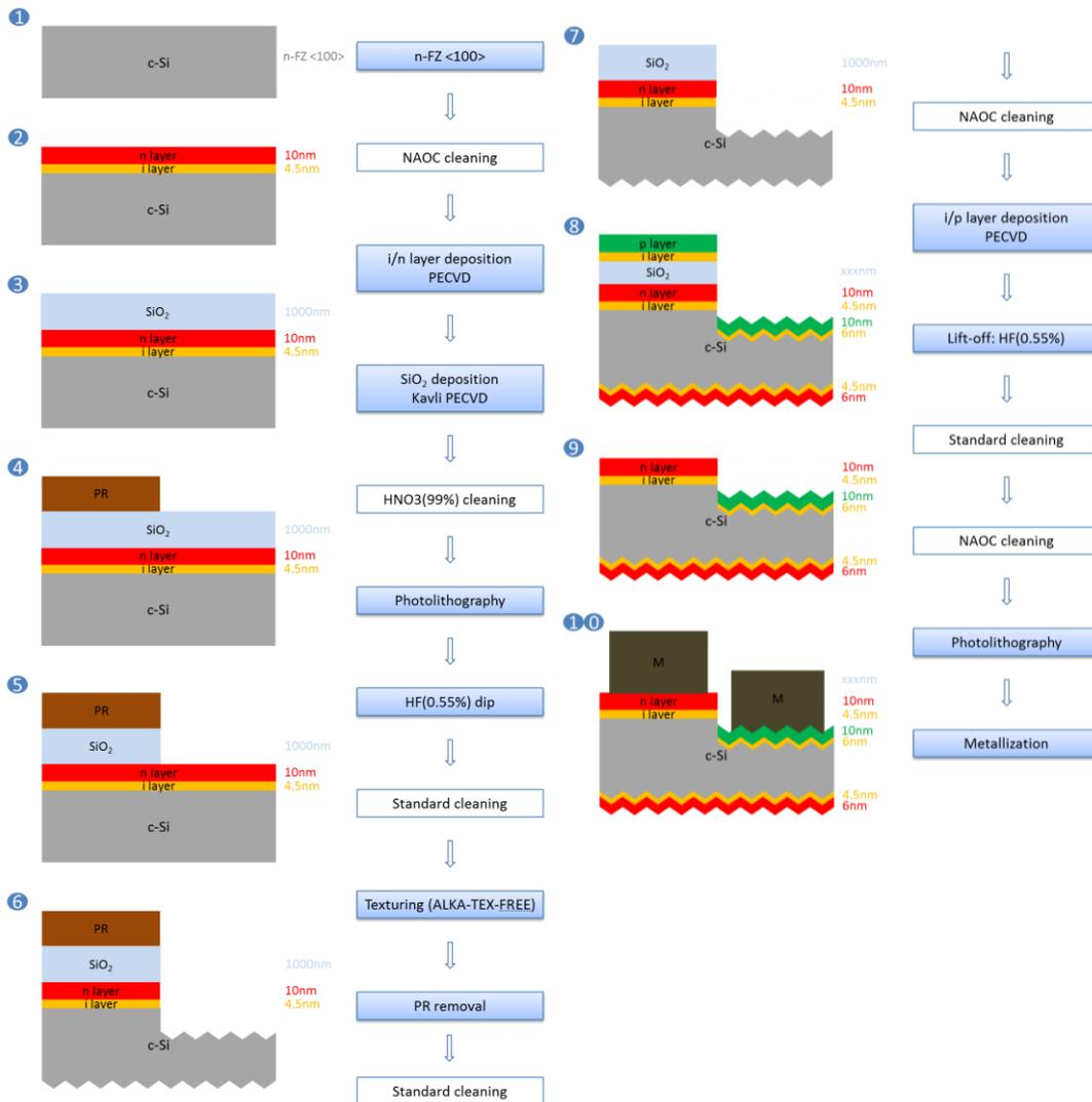
Figure 3.16 Fabrication flowchart of Approach 5
