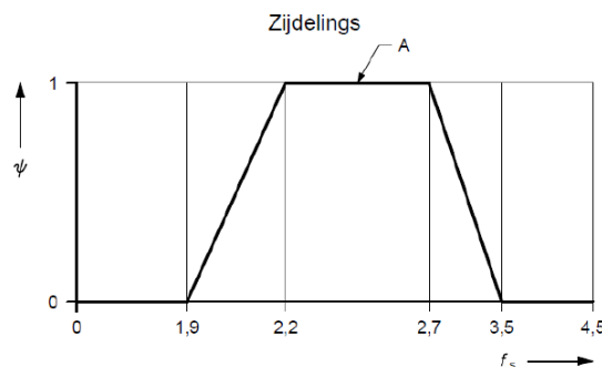
Figure E.5: Figure 5.7 of NA: Reduction factor of a single runner. A = first harmonic vibration.
