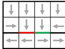
Figure 5.4: Example with an arbitrary layout where the compartment exit location choice influences results.
