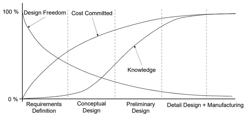
Figure 2.5: General design characteristics, from Cooper *et al.* [1]
