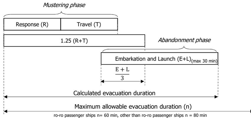
Figure 2.1: Performance standard according to IMO [16].
