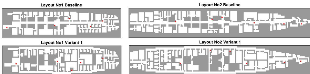
Figure 5.7: Project EGO layouts translated in MDP program, gray indicates walls, white are states, red is an exit state. Exits are number from aft to forward in ascending order.
