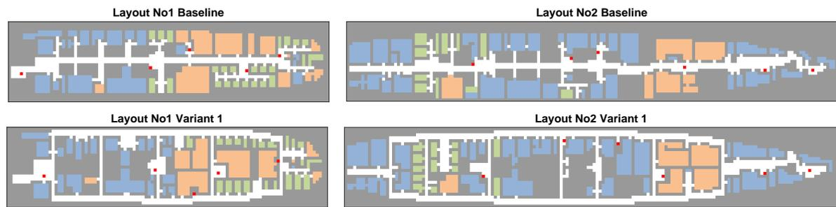
Figure 5.6: Assumed compartment type. Blue denote service spaces, orange denote public spaces, and green denote accommodation spaces.
