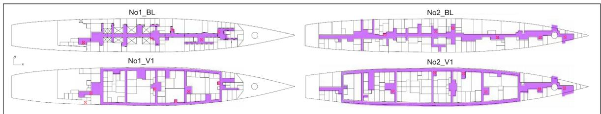
Figure 5.1: Example layout drawn in Rhinoceros with the passageway figure covered on top.
