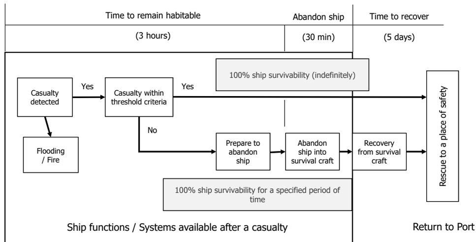
Figure 2.2: IMO framework - passenger ship safety. Adopted from [11].
