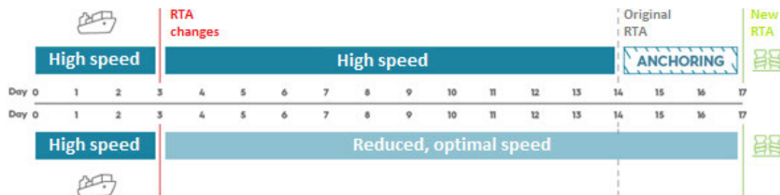
Figure 3.2: Clarification Just-In-Time concept. Source: IMO GIA (IMO GIA, 2019b), adapted by author.
