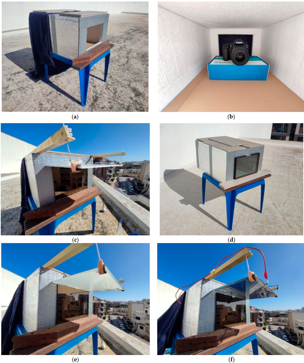
Figure 8. Selected photos of the testing setup. (a) Test box mounting on a secure base. (b) Luminance photometer within the test box. (c) Static opaque shading. (d) Unshaded configuration. (e) Solar-PDLC shading overhang (OFF state). (f) SPD shading overhang (OFF state).
