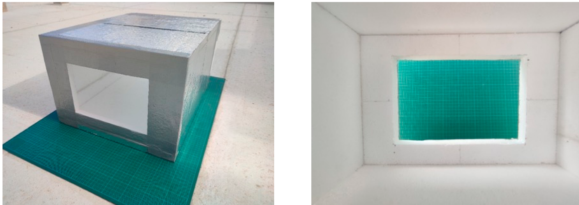
Figure 4. External and internal views of the scale model used for the luminance field experiments, prior to the placement of the light brown flooring.
