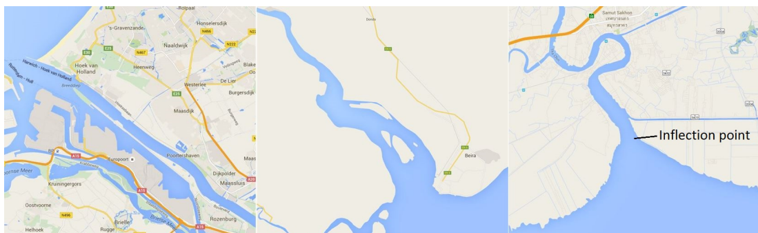
Figure 2.1: Left: prismatic estuary (Rotterdam Waterway), middle: funnel shaped estuary (Pungue), right: trumpet shaped estuary (ThaChin). (Google maps)
