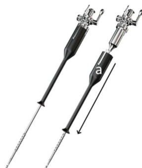
Fig. 2 The VeressPLUS (VN+) needle. Left, the additional safety sheet (a) that is in contact with the hand can dislodge. Right, conventional Veress needle versus VeressPLUS shows that overshooting is prevented because the needle sheet dislodges after puncturing the peritoneum, leaving the needle and stylet in place at the Optimal Insertion Depth (OID) without driving it further into the cavity [5]
