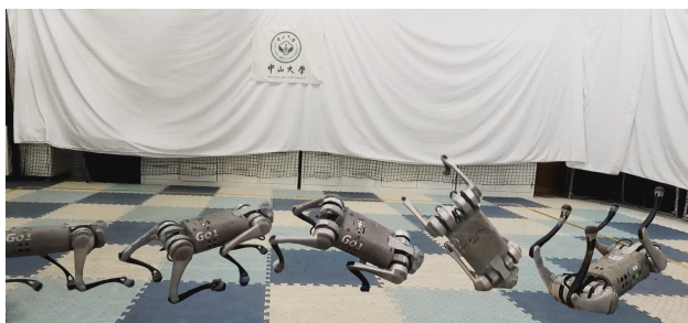
Fig. 3: Locomotion with only the CPG module. The robot is unable to maintain trunk stability and falls over as the front right foot gets stuck.
