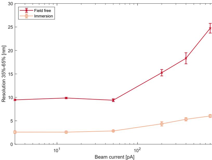
Figure 5.8: **Measured 35-65 electron beam resolution as a function of beam current for field-free and immersion SEM lens modes.** Immersion mode results in smaller spot sizes, which remain relatively constant with increasing current. The spot size in the field-free mode increases significantly with higher currents, 4x larger at below 50pA and up to 10x larger at 800pA.
