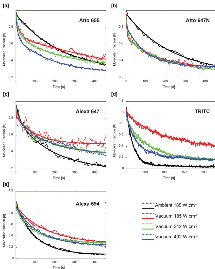
Figure 4.3: **Alexa 647, Alexa 594, and TRITC show lower photo-bleaching in a vacuum.** Photobleaching curves are represented as normalized molecular fraction vs time for (a)-(e) Atto 655, Alexa 647, Atto 647N, TRITC, and Alexa 594, respectively. Data was smoothed by a Gaussian weighted moving average filter and fit to a double-exponential function with an offset.
