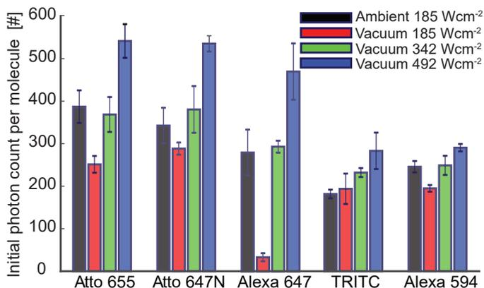
Figure 4.2: **TRITC retains photon count per molecule (at onset) in both ambient and vacuum environments.** Average photon count per molecule at onset for ambient (excitation: 185  $\text{Wcm}^{-2}$ ) and vacuum conditions (excitation: 185, 342 and 492  $\text{Wcm}^{-2}$ ). Error bars represent 95% confidence intervals.
