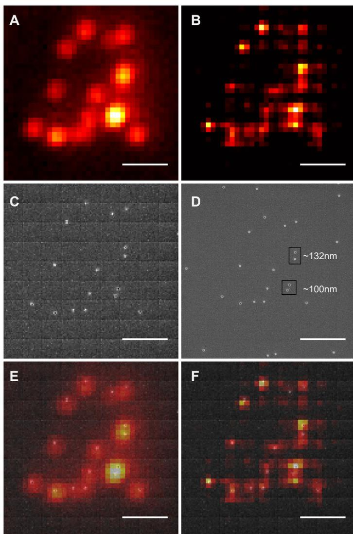
Figure 2.7: **~100nm eSRM localization accuracy on multiple fluorescent polystyrene microspheres.** (A) WF-FM image of a selected region of the microspheres sample, (B) eSRM super-resolution reconstruction of the same area, (C) RT-SEM image, (D) post-eSRM high-resolution SEM image, and (E) the final CLEM overlay with the WF and (F) SR image. Inset (D) depicts sub-diffractive bead twins' center-to-center spacing. Scale bar 1 $\mu$ m.
