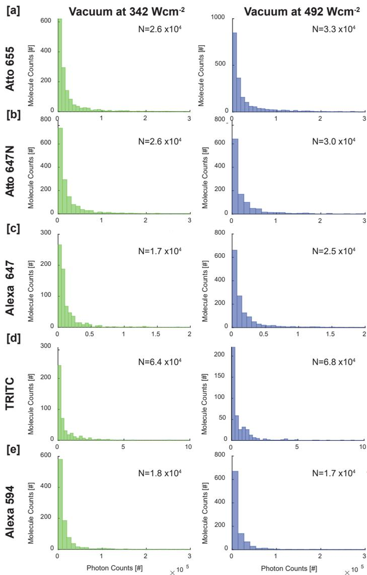
Figure 4.5: **TRITC shows ~3-fold increase in mean photon yield under vacuum.** Histogram of molecule versus photon counts under vacuum conditions at  $342 \text{ Wcm}^{-2}$  and  $492 \text{ Wcm}^{-2}$  excitation intensity. (a)-(e) Atto 655, Alexa 647, Atto 647N, TRITC and Alexa 594 respectively. Legend denotes the mean photon yield as obtained from a single exponential distribution fit. Note: TRITC had a 2250s acquisition time, whereas the remaining dyes were measured for 450s.
