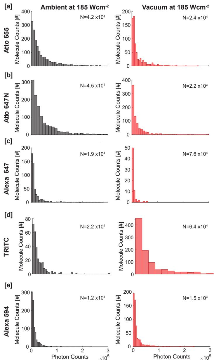
Figure 4.4: **TRITC shows ~3-fold increase in mean photon yield under vacuum.** Histogram of molecule versus photon counts under ambient (black) and vacuum (red) conditions at 185 Wcm<sup>-2</sup> excitation intensity. (a)-(e) Atto 655, Alexa 647, Atto 647N, TRITC and Alexa 594 respectively. Legend denotes the mean photon yield as obtained from a single exponential distribution fit. Note: TRITC had a 2250s acquisition time, whereas the remaining dyes were measured for 450s.
