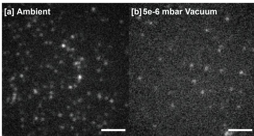
Figure 4.1: **Atto 655 shows reduced emission intensity and fewer fluorescent molecules under a vacuum.** Atto 655 molecules at (a) ambient and (b) vacuum ( $5\times 10^{-6}$  mbar) conditions with 638nm excitation wavelength and  $185\text{ Wcm}^{-2}$  excitation intensity. Scale bar  $5\mu\text{m}$ . Images were contrast-scaled for visibility.
