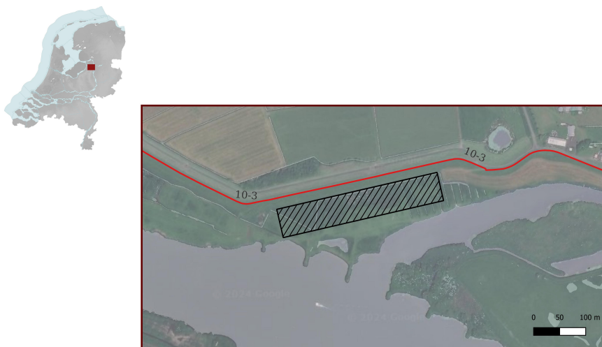
Figure 5.1.: Dike [trajectory 10-3] along the river IJssel, where the black coloured raster shows the potential forest area and the red line indicates the primary dike.
