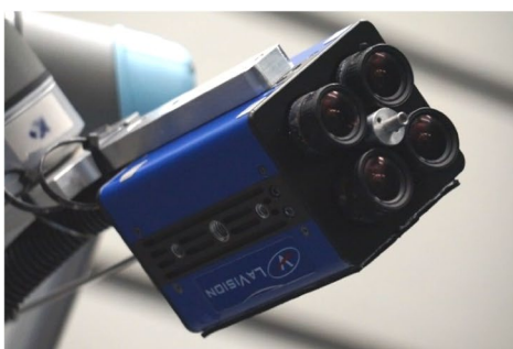
Fig. 5 Robotic PIV measurement setup; left: CVV module and right: operating principle of the coaxial velocimeter, showing cameras (blue), field of view (grey) and laser illumination (green) provided by
