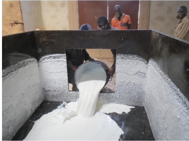
Figure 30. The chemicals are mixed and poured in a container to produce latex foam
