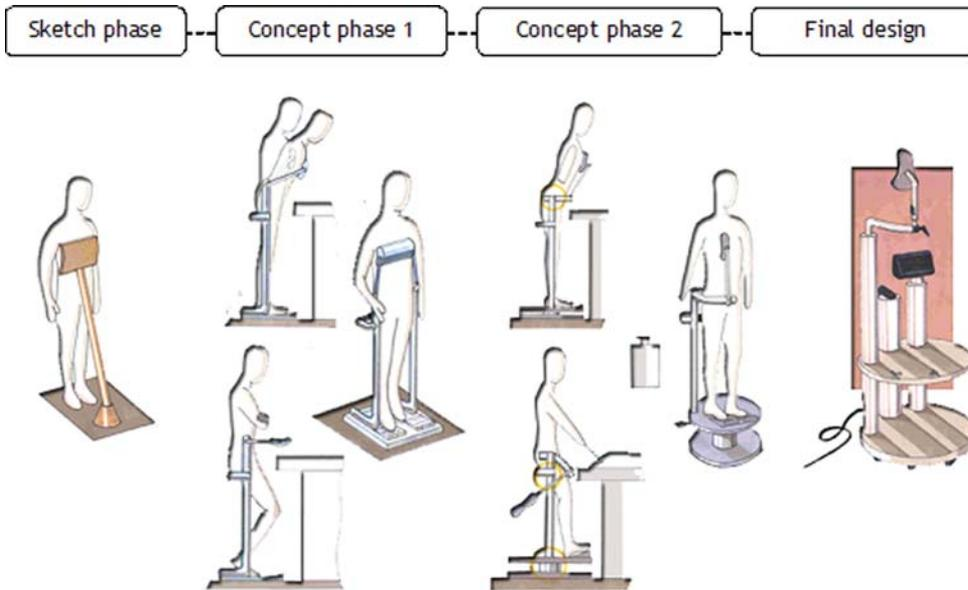
**Fig. 1.** Design process for the ergonomic surgeon's body support.
