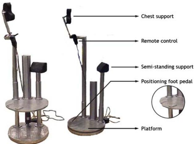
**Fig. 2.** Prototype of the ergonomic surgeon's body support.
