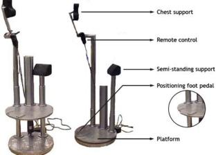
Fig. 2. Prototype of the ergonomic surgeon's body support.
