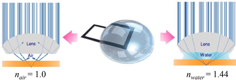
Figure 1.5: Schematic of a liquid immersion droplet in photolithography where n is the refractive index.
