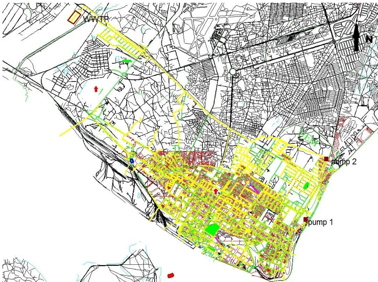
Figure 6: AutoCAD drawing of the sewer network of Maputo. Pumping stations one and two and the WWTP are indicated. Source [27].
