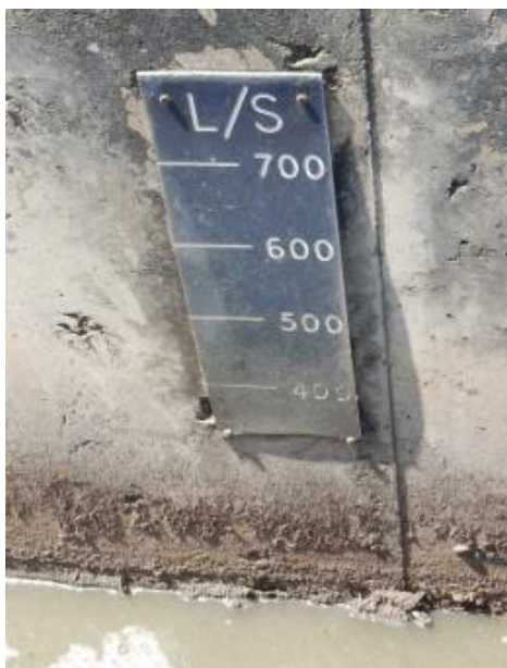
Figure 3: Broken level meter. The meter would convert directly the water height into water flow (L/s).
