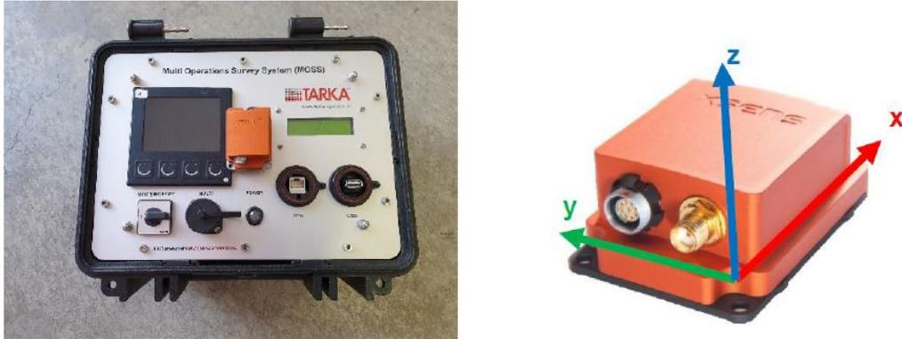
Figure 5.4: A picture of the jacket sensor and the proposed axis system [13]
