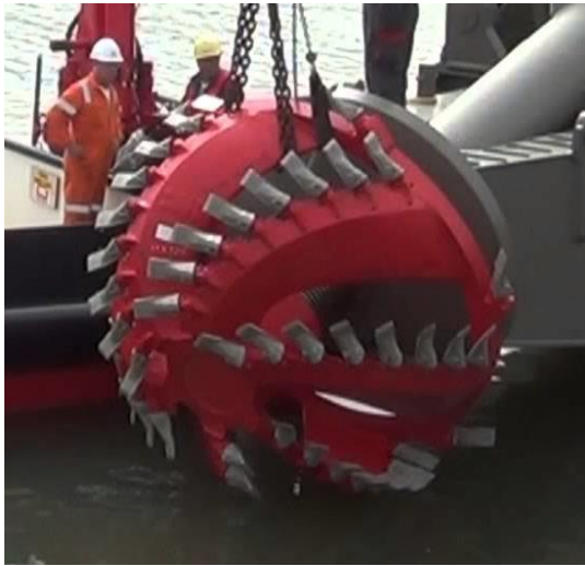
Figure 3-12, Typical Cutter head (Royal IHC, MTI)
