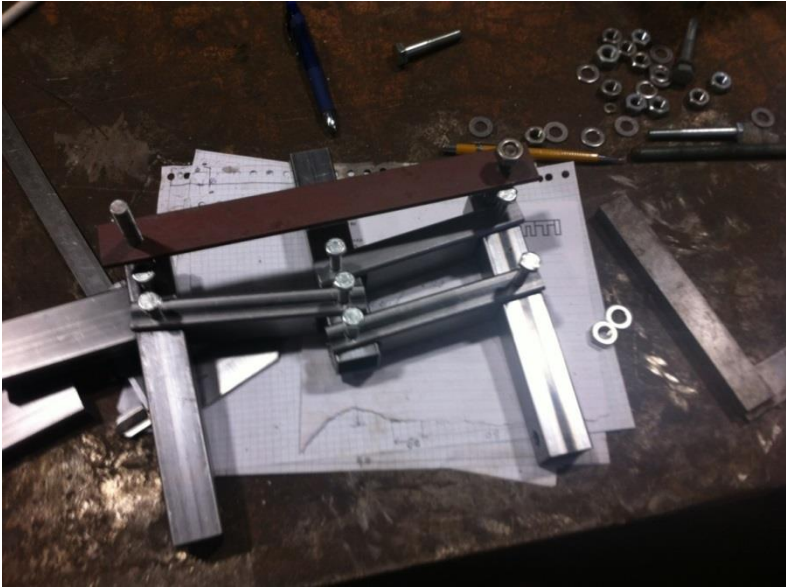
Figure 5-4, Added top tension element
