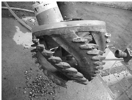
Figure 7.4: The crown cutter head and the results of the tests for mixture velocities of 2.5 m/s and 4.0 m/s
