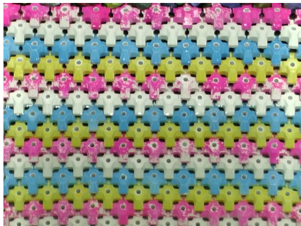
Figure 1.2 Regular placement of the Xbloc+
