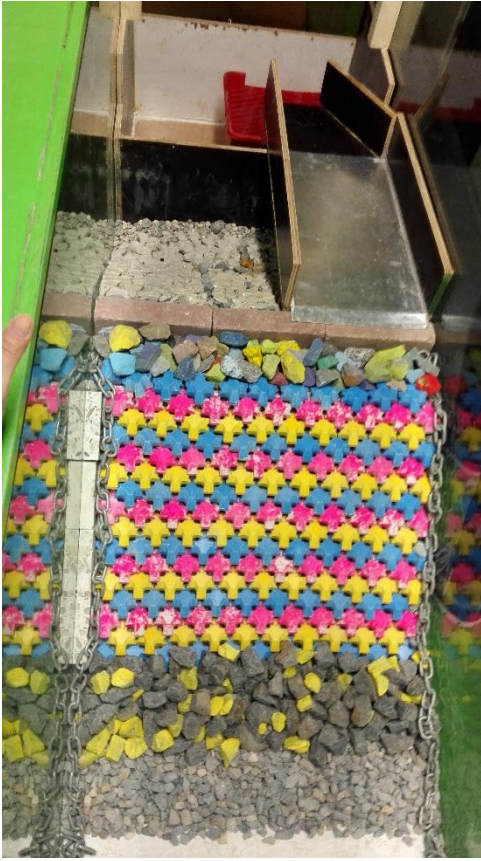
4 Top view (slope 3:4 initial blocs)
