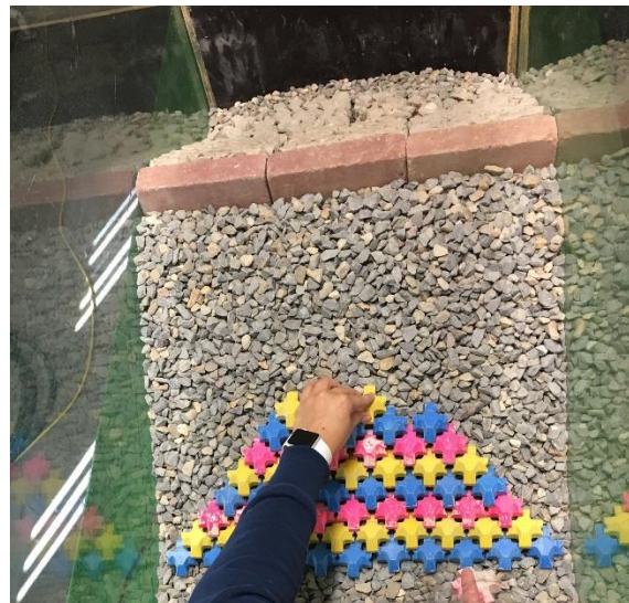
9 Placement of the concrete unit
