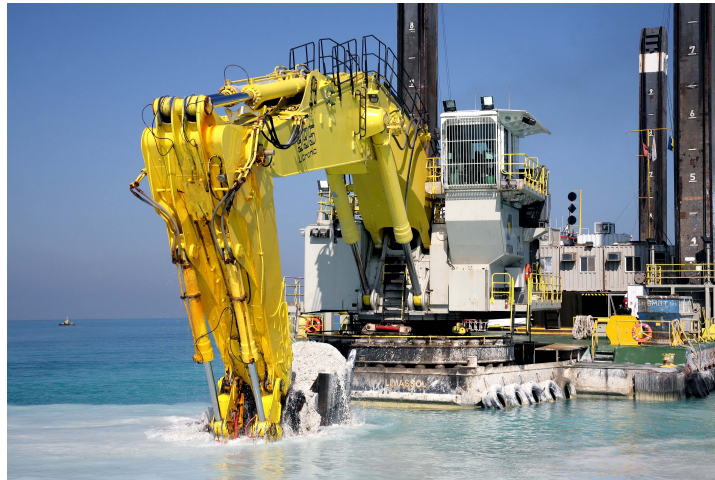
Figure 7.1: Backhoe dredger (source: http://www.boskalis.com/ )
