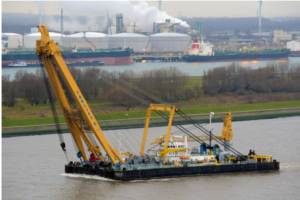
Figure 7.4: Floating sheerleg, Taklift 4 (source: http://www.shipspotting.com/ )
