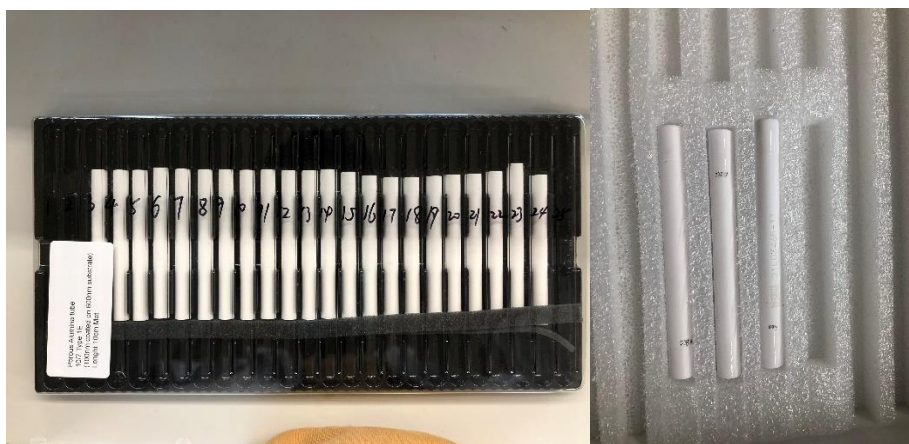
Figure 4. Photos of alumina membranes from coorsTek (left) and Inopor GmbH (right)
