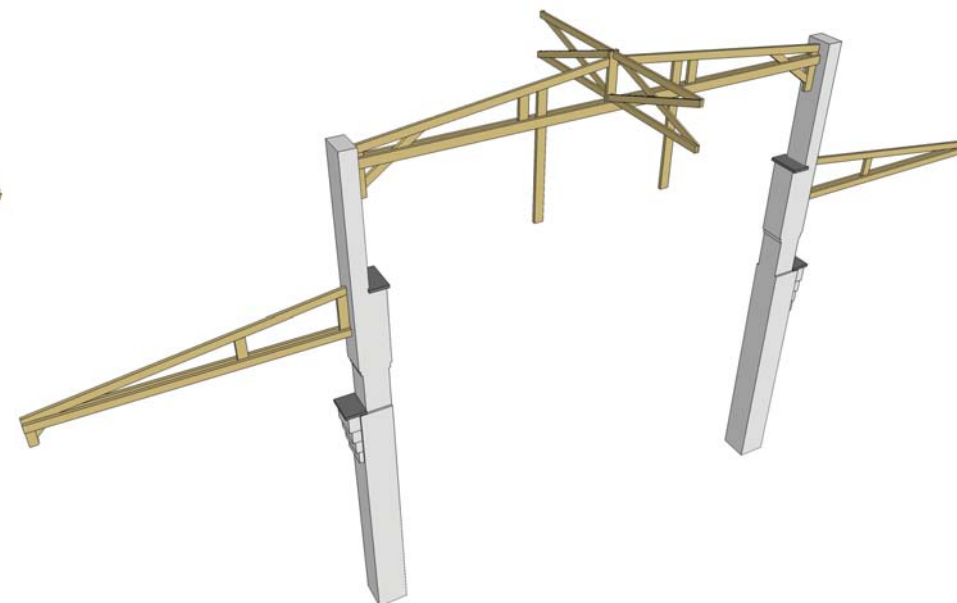
wooden truss systems - main nave and apsis are not directly connected, they rest individually on the central pillars.
