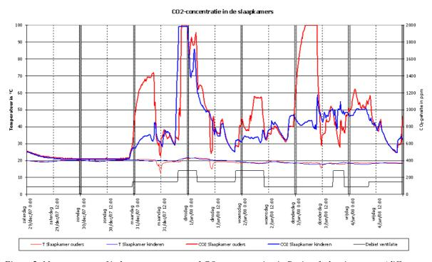
Figure 2. Measurements of indoor temperature and  $CO_2$  concentration in Project 1 sleeping rooms (different scenarios during a winter period). Measurements by G. De bruyn, Cenergie cvba, presented on PassiveHouse 2008, Brussels. The lower curve represents the ventilation setting in three possible positions.
