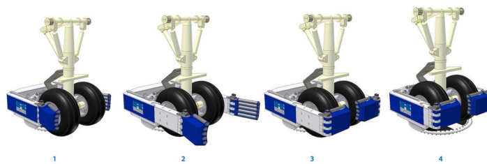
Figure 2.2: The clamping mechanism between the NLG and TaxiBot [40]. 1 & 2: The nose wheel enters the clamping mechanism. 3 & 4: The nose wheel is clamped and lifted and is able to rotate freely.
