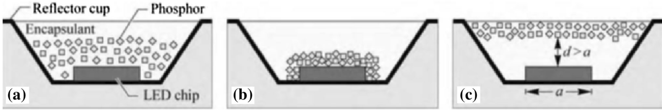
Fig. 1. Schematics of (a) proximate phosphor distributions, (b) conformal proximate phosphor distributions, and (c) remote phosphor distribution. 4
