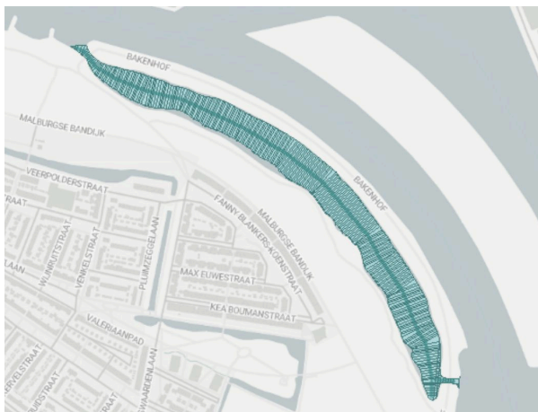
Figure 34. Perpendicular lines to centerline clipped to Bakenhof side channel polygon (own figure)
