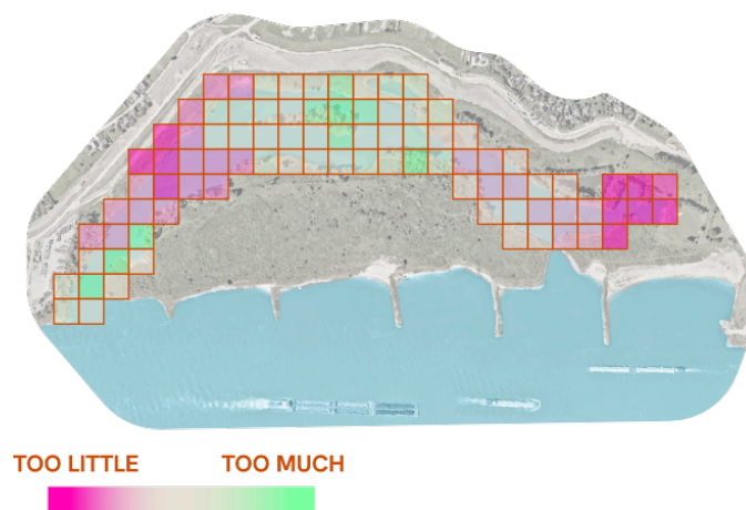
Figure 13. Example of an error map, in which pink represents areas where the prediction is lower than reality, and green represents areas where the prediction is higher than reality (own figure)
