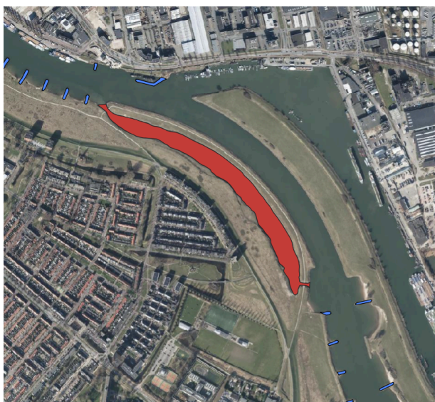
Figure 28. Groynes (blue) near Bakenhof side channel (red) (own figure)
