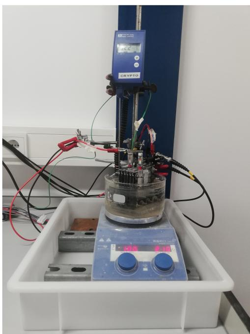
Figure 3.1: The experimental setup includes the cell, hot plate, water bath, and electrical connections.
