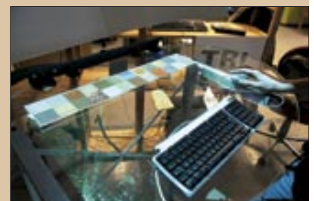
Projected images can be used to flexibly try out textures, buttons, displays, etc. on foam models.
