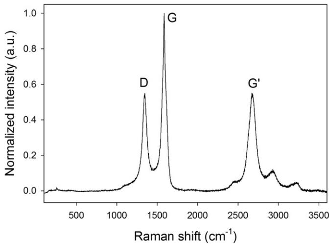
Fig. 4. Raman spectrum of CNT grown on test samples using the same growth recipe. The intensity is normalized to the G-band.
