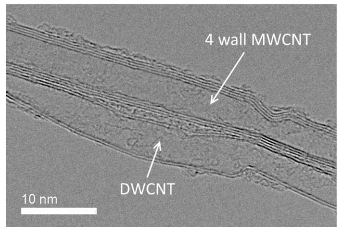
**Fig. 3.** Typical TEM image of CNT grown on ZrN using the growth recipe used in this work.
