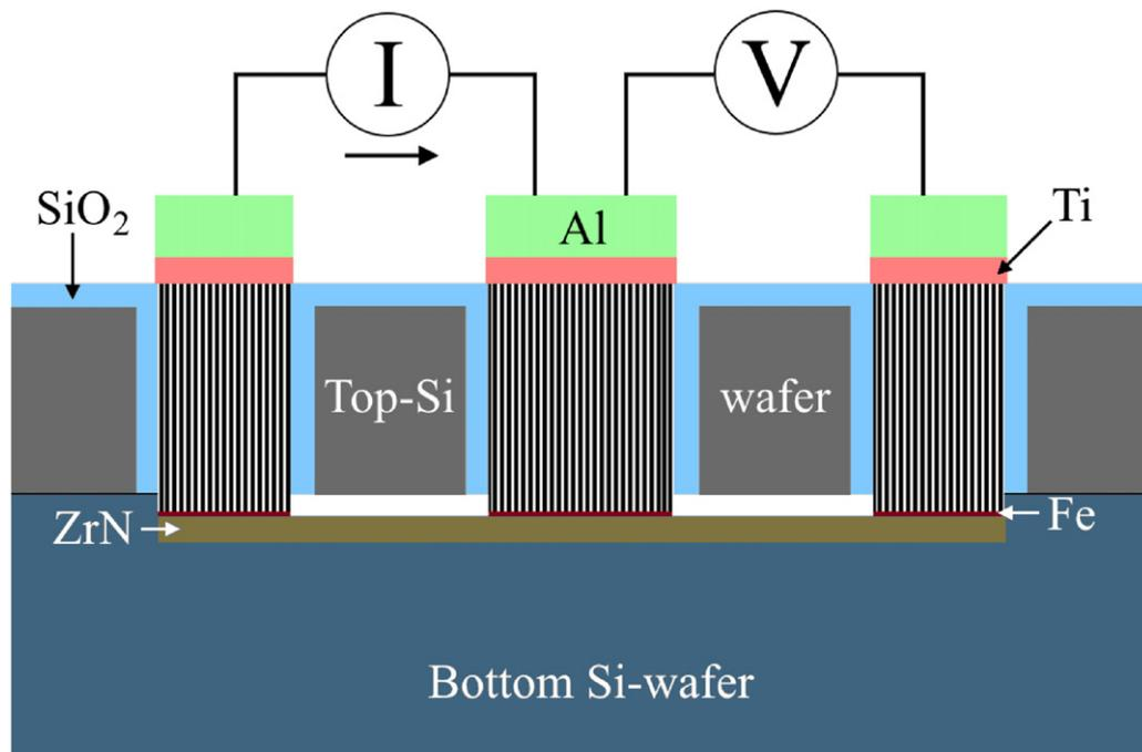
Fig. 1. Schematic cross-section of the 4-point probe measurement structure fabricated using the described method.
