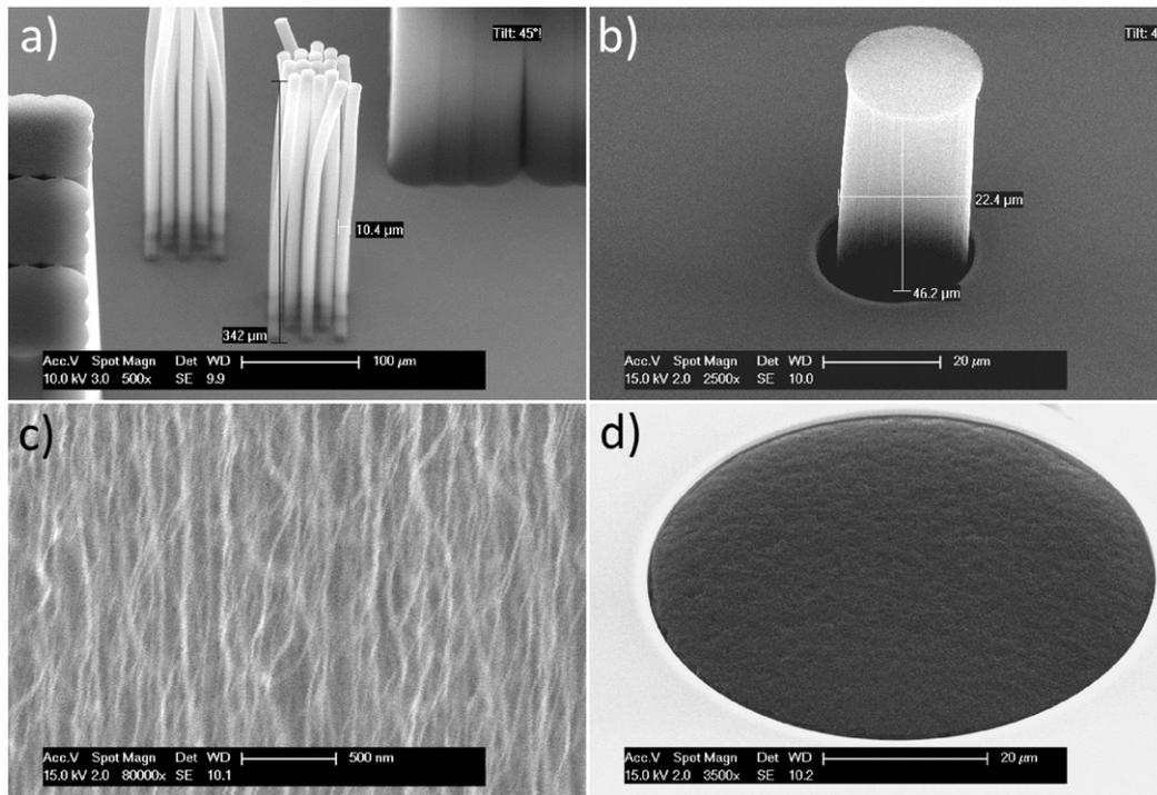
**Fig. 2.** SEM images of CNT grown on ZrN using 0.8 nm of Fe: a) high-aspect ratio bundles; b) bundle with AR 15 inside TSV opening; c) close-up of CNT bundles indicating alignment and density; d) 60  $\mu\text{m}$  CNT bundle grown inside a 300  $\mu\text{m}$  deep through-silicon hole.
