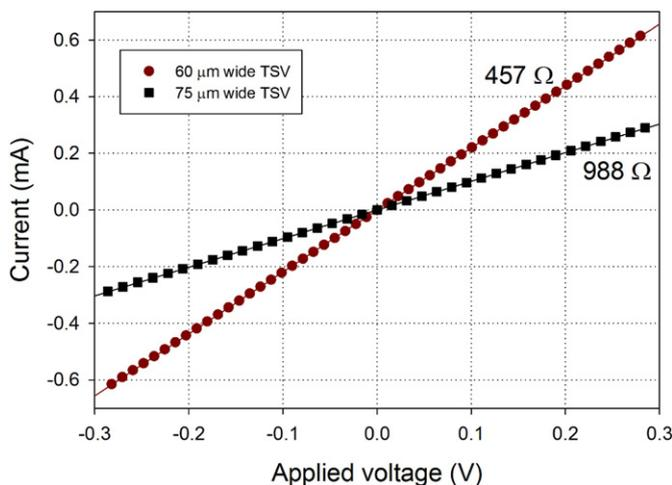
Fig. 5. I–V characteristics of CNT TSVs with diameters of 60  $\mu\text{m}$  and 75  $\mu\text{m}$ , and length of 300  $\mu\text{m}$  (AR 5 and 4, respectively), measured using 4-point probe structures.
