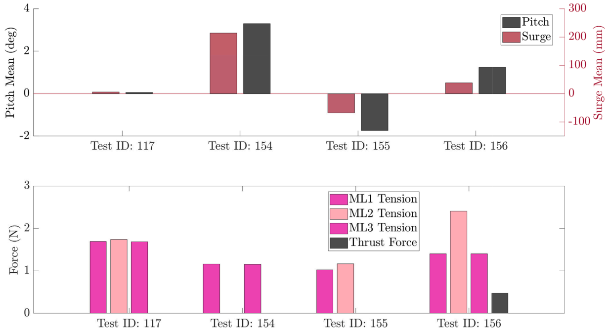
Fig. 26. Surge, pitch, mooring lines and thrust mean values in different ALS conditions.
