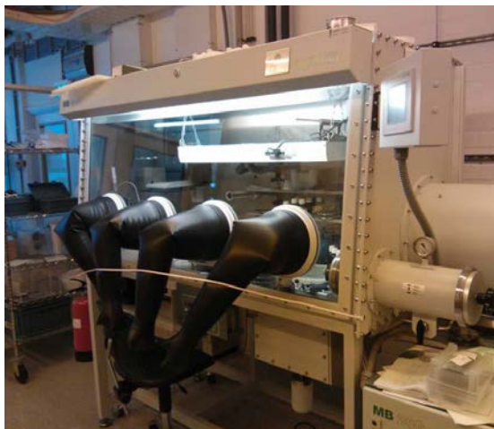
Figure 2.3 Photo of the glove box, used for the processing of 100% CPS and the liquid-Si solution in an oxygen- and water-free environment.
