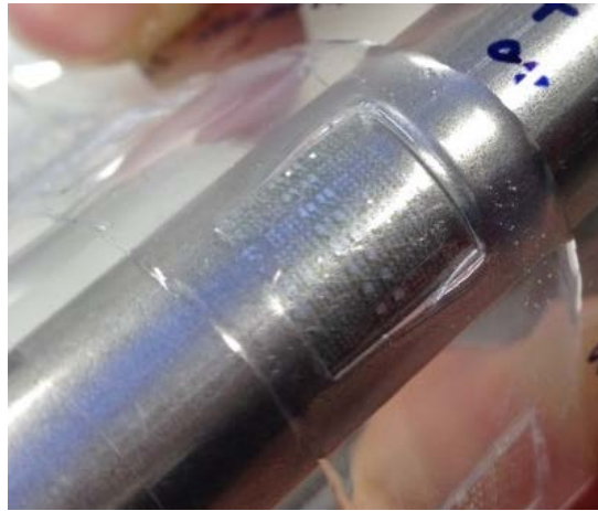
Figure 5.7 SG-TFTs bend for reliability measurement on PEN foil
