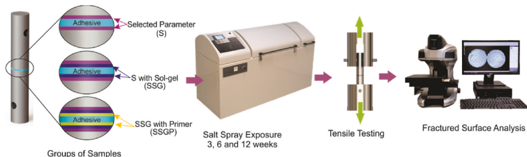
Fig. 3. Adhesive bond quality assessment sequence after salt spray exposure.
