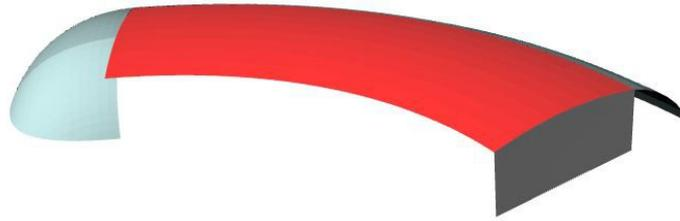
Illustration 4.17: Supports in transverse direction for cylindrical roof
