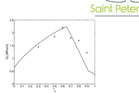
*Figure 13* Model fit to the data of Chabert et al. (2012) using only the water-saturation-dependent function  $F_2$ . *Parameter values are* fmmob = 5.5, fmdry = 0.550,  $f_g^* = 0.65$ .
