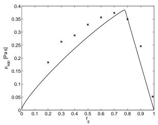
**Figure 9** Model fit to the data of Moradi-Araghi et al. (1997) using only the water-saturationdependent function  $F_2$ . Parameter values are fmmob =  $5.57 \cdot 10^3$ , fmdry = 0.336, fg<sup>\*</sup> = 0.78
