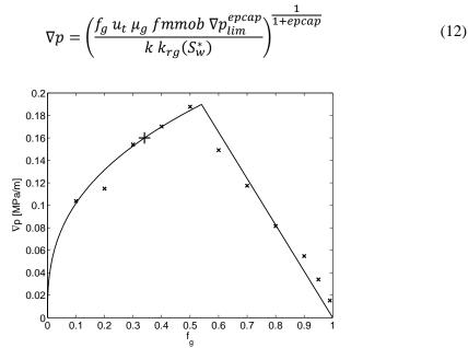
**Figure 6** Model fit to data of Ma et al. (2012) including the capillary-number-dependent function  $(F_5)$  in the low-quality regime. Data points in the low- and high-quality regimes are shown by crosses. The solid line shows the model fit. The '+' sign is the chosen value of  $(f_g^+, \nabla p(f_g^+))$ .
