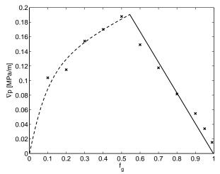
*Figure 4* Data of Ma et al. (2012). Data points are shown as crosses. Initial, hand-drawn, fits to data in low- and high-quality regimes are shown as a convex, dashed curve and a solid straight line respectively.
