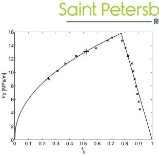
**Figure 8** Model fit to the data of Alvarez et al. (2001) including the capillary-number-dependent function  $F_5$ . Parameter values are fmmob =  $6.63 \cdot 10^5$ , fmdry = 0.311, epcap = 1.13, fmcap =  $2.46 \cdot 10^{-5}$ . The '+' sign is the chosen value of (fg<sup>+</sup>,  $\nabla p(fg^+)$ ).
