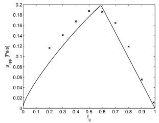
**Figure 11** Model fit to the data of Moradi-Araghi et al. (1997) using only the water-saturationdependent function  $F_2$ . Parameter values are fmmob =  $3.28 \cdot 10^3$ , fmdry = 0.385, fg<sup>\*</sup> = 0.59
