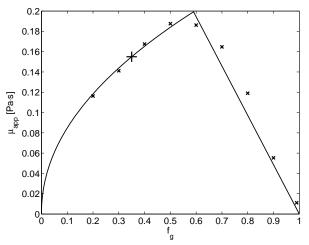
**Figure 12** Model fit to the data of Moradi-Araghi et al. (1997) including the capillary-numberdependent function  $F_5$ . Parameter values are fmmob =  $1.86 \cdot 10^4$ , epcap = 1.08. The '+' sign is the chosen value of  $(f_g^+, \mu_{app}(f_g^+))$
