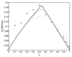
*Figure 14* Effect of epdry on model fit to data of Ma et al. (2012) excluding for simplicity the capillarynumber-dependent function ( $F_5$ ) in the low-quality regime. Curves correspond to the following values of epdry: 100,000, 10,000, 1,000, 100.
