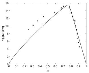
**Figure 7** Model fit to the data of Alvarez et al. (2001) using only the water-saturation-dependent function  $F_2$ . Parameter values are fmmob =  $4.27 \cdot 10^4$ , fmdry = 0.311,  $f_g^* = 0.775$
