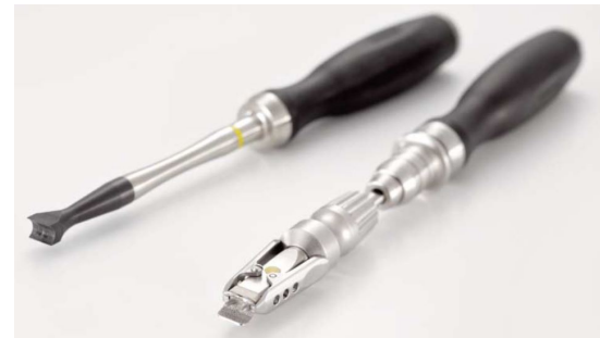
(b) The proximal impactor (left) and the positioner (right) used for insertion of the test prosthesis.
