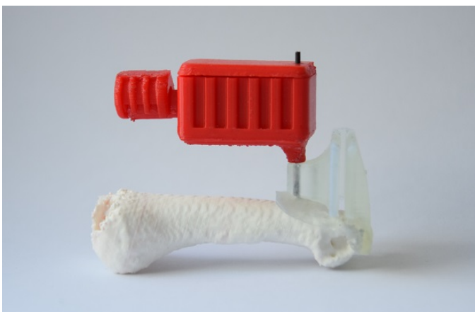
Figure 4.8: A photograph from the side of the Patient Specific Surgical Guide (PSSG) (transparent) on top of an 3D-printed proximal phalanx of the middle finger. The PSSG is constrained to the bone by a pin and a clamp (red).
