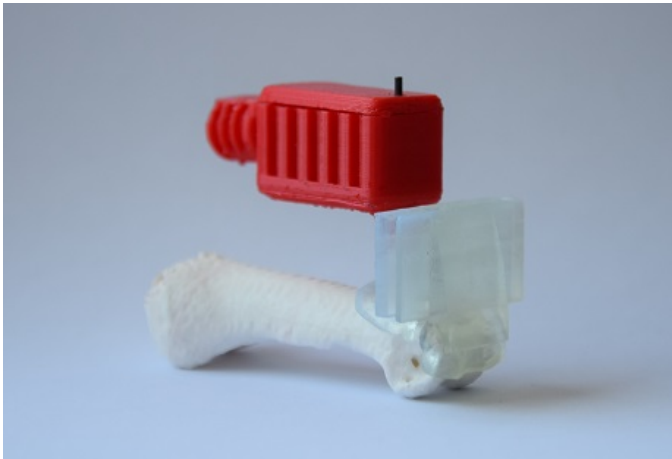
Figure 4.7: Photograph of the Patient Specific Surgical Guide (PSSG) (transparent) on top of an 3D-printed proximal phalanx of the middle finger. The PSSG is constrained to the bone by a pin and a clamp (red).
