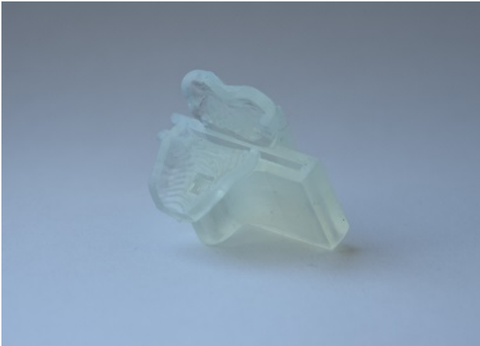
Figure 4.3: Photograph of the patient specific surgical guide turned upside-down. The negative mold of the head of the proximal phalanx, the channel through which a pin is drilled and the slot to guide the saw-blade are clearly visible.
