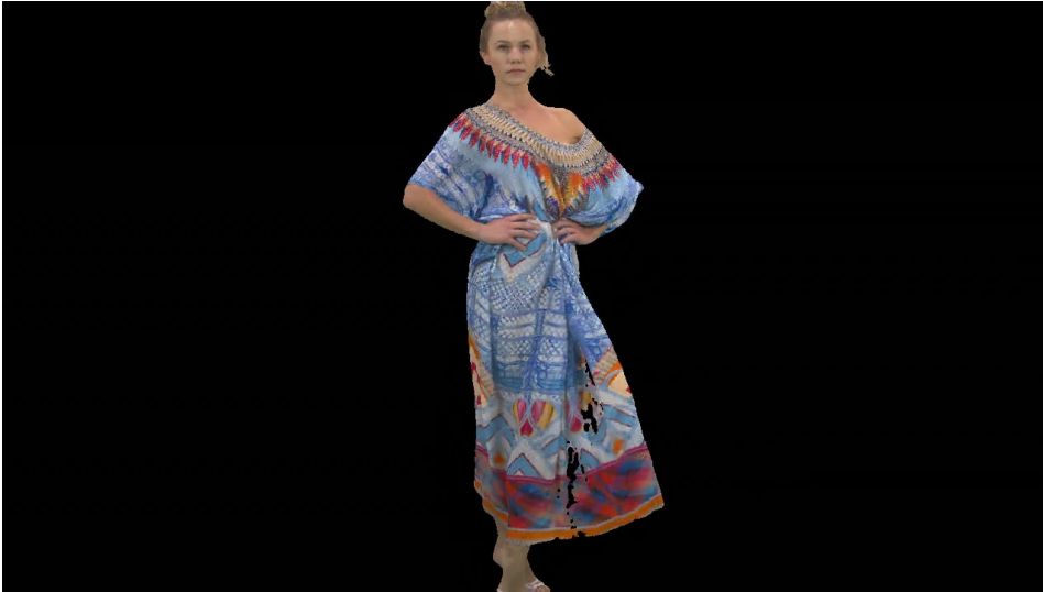
Figure 5.1: Compression artifact in the decoded stream introduced by inter prediction
