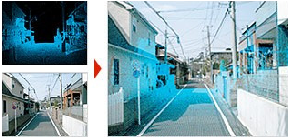
Figure 2.9: Map creation where point clouds captured by laser scans are overlaid over camera images [13]
