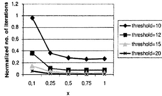
Fig. 4. Normalized mean number of iterations versus phase shift variance parameter  $x$  for 8-carrier OFDM system and different threshold levels, simulated with random phase updating algorithm of Fig. 2(A).
