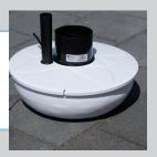
Hypothesis 8 – It is not possible to conclude on this hypothesis. The trap performed poorly against the Suna-Trap. The canopy used in this concept featured a pattern of larger holes than that of the Suna-Trap and it was later found that this is detrimental to performance. It is therefore not possible to conclude on whether the absence of an inlet pipe inhibits performance or not.
