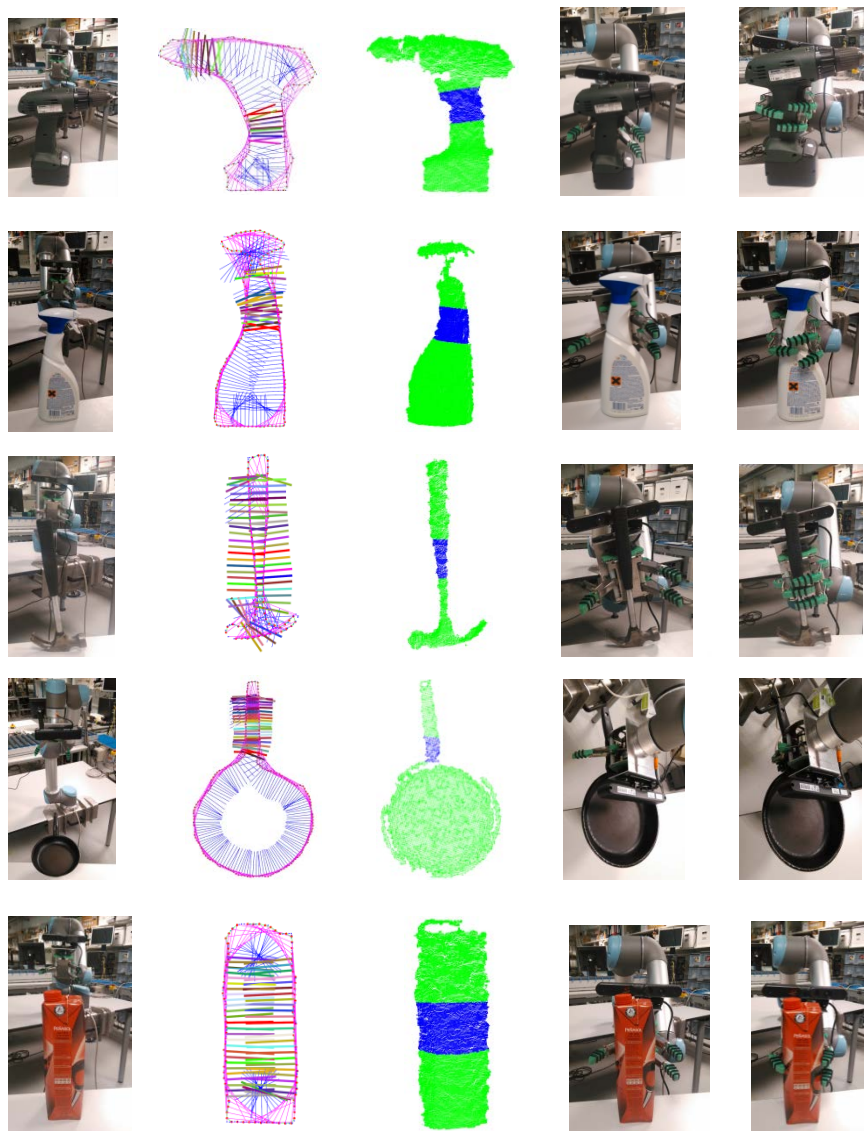
Figure 4.20: Snapshots from the experiments: First column is the initial state of the robot and the target objects. Second column is the result of grasping computation. Third column shows the grasp area on the point cloud of the target object. Fourth column shows the gripper arriving at grasping point. Fifth column shows objects grasped by gripper.
