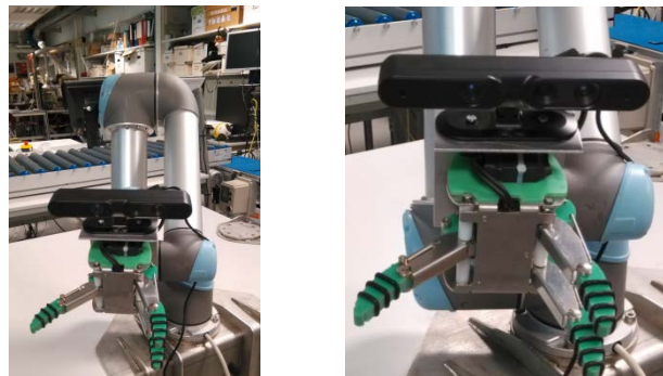
Figure 4.19: Experiment setup. A Lacquey under-actuated gripper and an Asus Pro Live sensor are installed at the end of the Universal arm (UR5).
