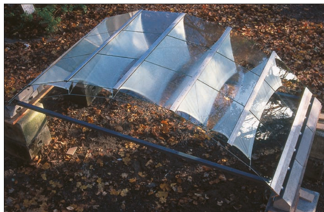
Fig. 61: 1:4 Model solar shading intergrated glass structure (Wurm, 2007)
