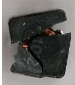
Figure 6. Broken inductor by the pneumatic hammer
