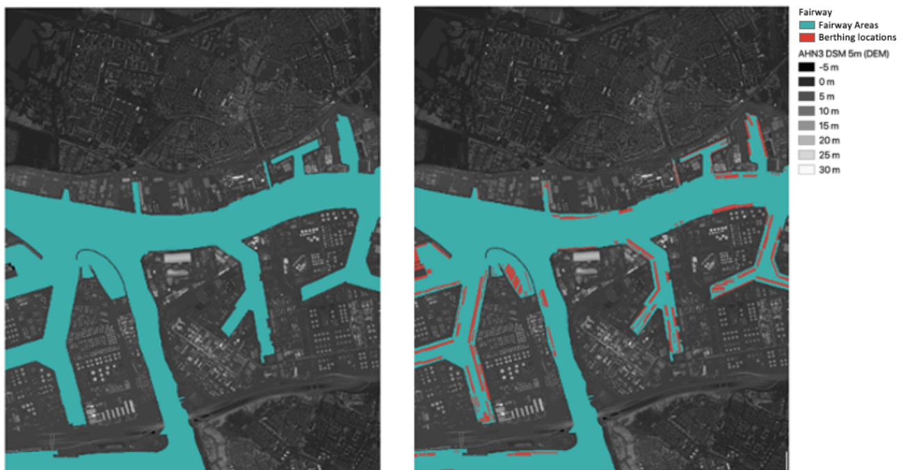
Figure 5-3 DEM Files for viewshed-analysis. Left) Static DEM, Right) Dynamic DEM.
