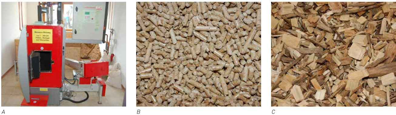
FIG. 4.2 Biomass boiler (A), wood pellet (B) and wood chips (C) (Image source courtesy 3N e.V.)
