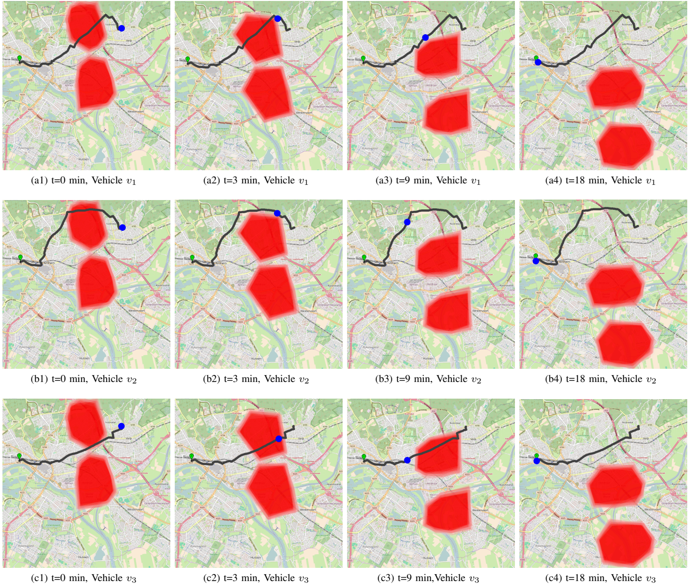
Fig. 14: Snapshots of routes calculated for 3 vehicles (in blue circle) with different r_{max} . The vehicles have the same source and destination points. The shapes and positions of the obstacles (in polygons) are the same in the three simulations, and change as the vehicles are moving towards the destination. (a) Vehicle v_1 , r_{max} = 0 min. (b) Vehicle v_2 , r_{max} = 2 min. (c) Vehicle v_3 , r_{max} = 7 min.
