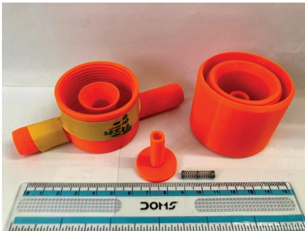
FIGURE 7: 1st generation design version of the RMT device showing valve plunger, valve body, spring, and valve cap for adjustment.
