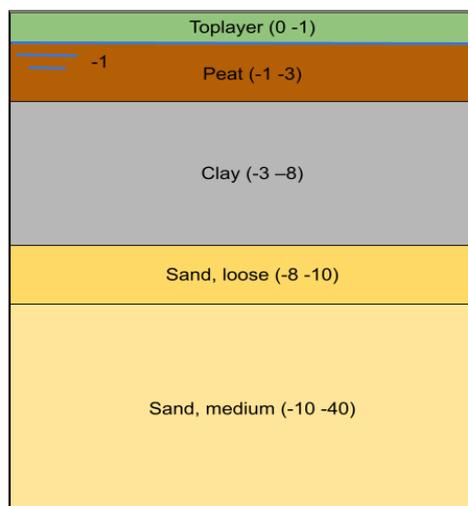
Figure 22: Schematic subsurface layering
