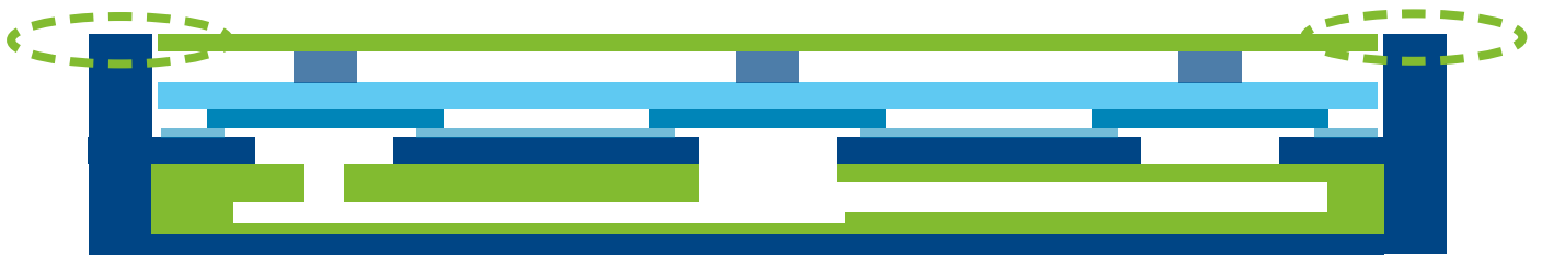
Figure 62, Model 3 with a metal top layer, partially open speaker chamber and thicker outer edge
