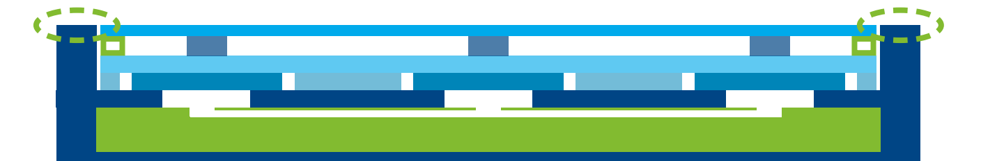
Figure 66, Model 7 with a foam suspension edge, partially filled speaker chamber and thinner outer edge
