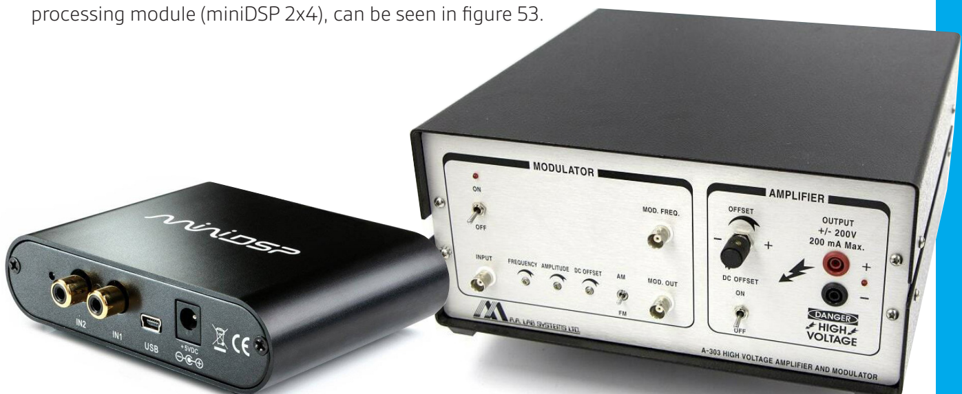
Figure 53, The digital sound processing device (left) and one of the used amplifiers (right)
