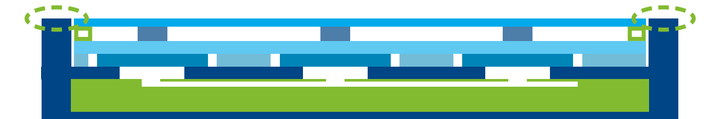
Figure 67, Model 8 with a foam suspension edge, partially filled speaker chamber, different layout, number of piezoelectric discs and thinner outer edge
