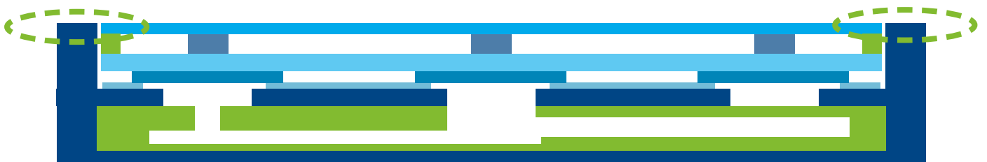
Figure 63, Model 4 with a adhesive ridge edge, partially open speaker chamber and thicker outer edge
