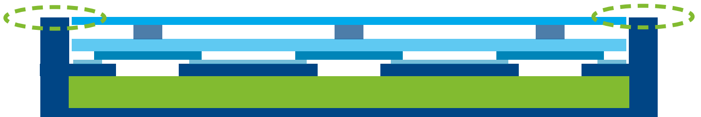
Figure 65, Model 6 with a free floating top layer, fully filled speaker chamber and thicker outer edge
