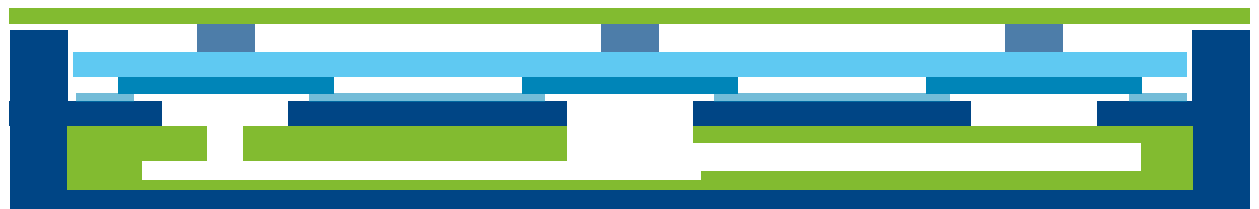
Figure 64, Model 5 with a free floating top layer, partially open speaker chamber and no outer edge
