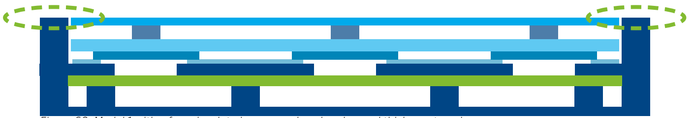
Figure 60, Model 1 with a foam insulated open speaker chamber and thicker outer edge
