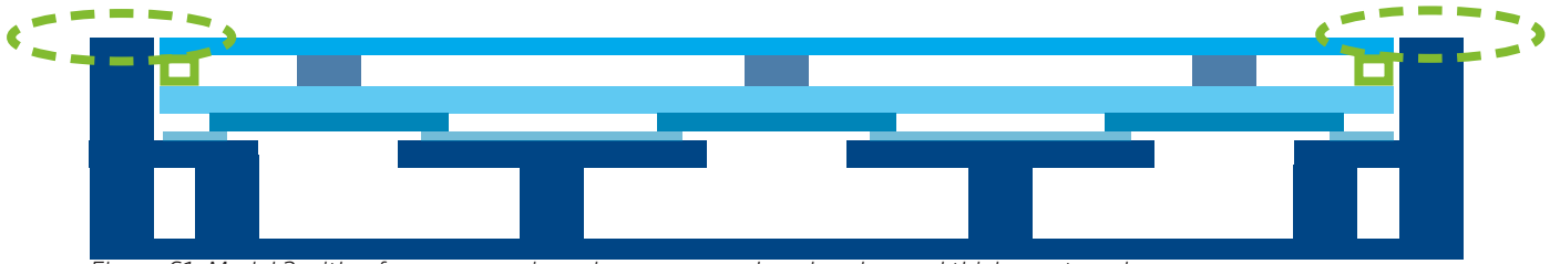
Figure 61, Model 2 with a foam suspension edge, open speaker chamber and thicker outer edge
