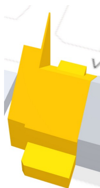
Figure 9. An example of a model with a “screen”. This model has an RMS of 0.04 m, and a maximum model-to-point distance of 6.1 m.
