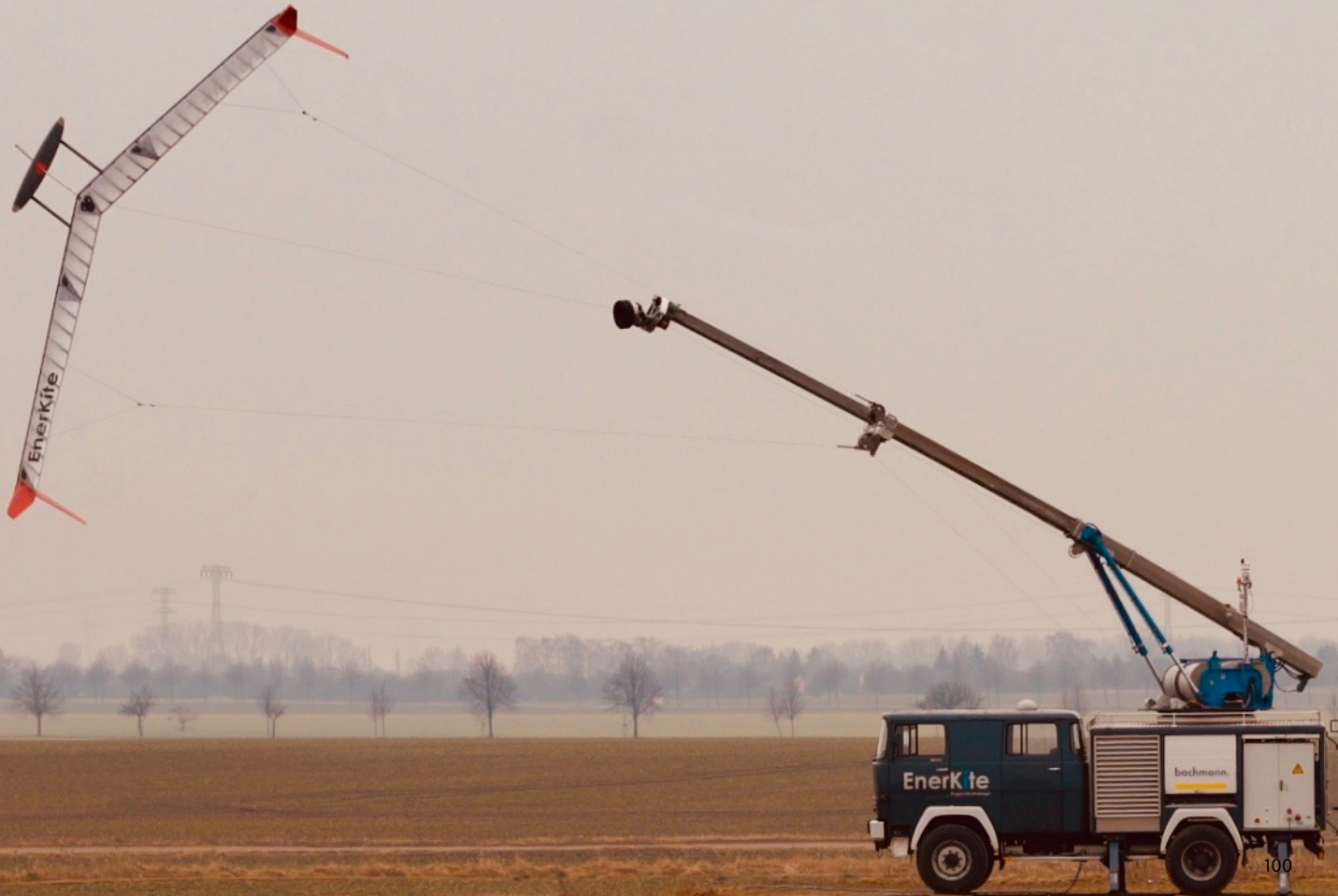
Rotational launch mechanism of Enerkite (25 September 2018)
