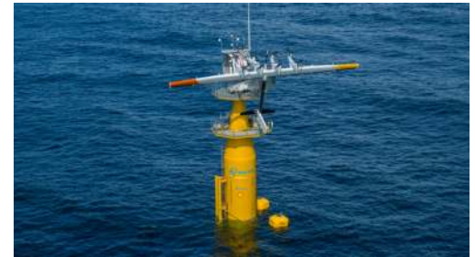
The Makani energy kite rests on its base station atop a floating platform during Makani's first offshore test campaign. August 2019.
