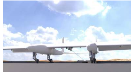
Tether-arrested landing, showing aircraft landing on a platform with tailored arresting system.
